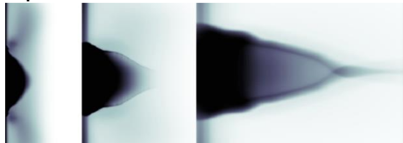
Experimental x-ray radiographs showing collimation of jets (Yurchak et al.)
